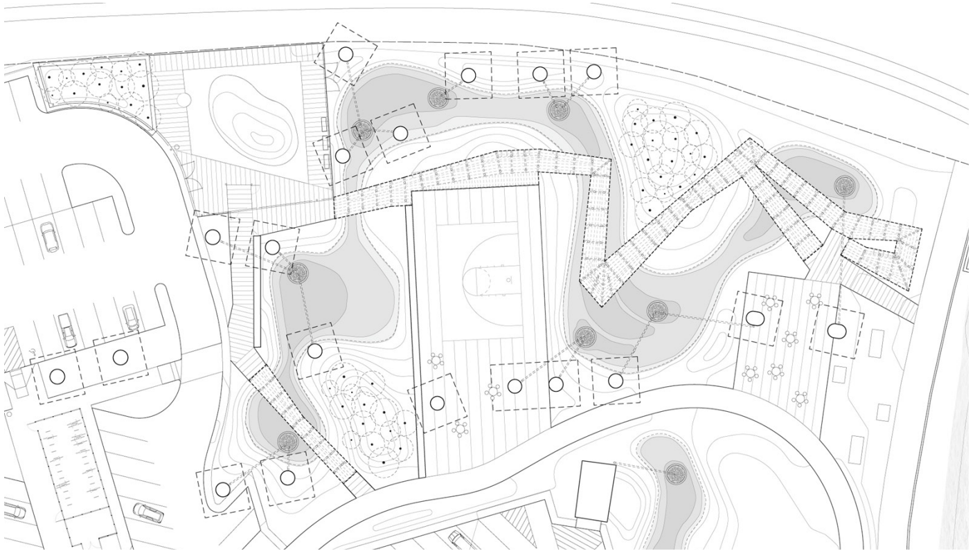
Figure 4: New ordering frame of mobility, planting, lighting, and recreation plates for storm-water management landscape at Infra-Space 1 in Boston, MA, drawings: Landing Studio
